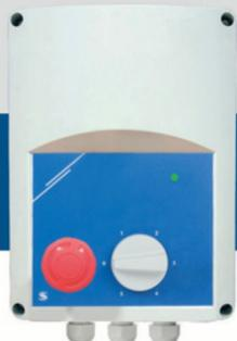
The SER-1 series of transformer fan speed controllers regulate the rotational speed of single-phase voltage controllable motors by varying the output voltage. They are equipped with an auto-transformer and control the speed manually in five steps. The technology used provides a regulated output voltage with a perfect sinusoidal shape. The controllers feature an emergency button for smoke extraction.
